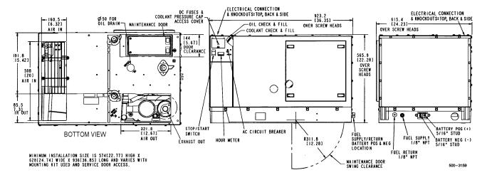
**Note:** This outline drawing is provided for general reference only and is not intended for design or installation. For more information see Operation and Installation manuals or obtain drawing 500-3159 and wiring diagram from your distributor/dealer.
